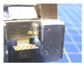
The starting handle can be fabricated using part 31 and a small length of .9mm and 1.5mm brass rod. Solder a 10mm length of .9mm brass rod to the slim side of part 30 and a 13mm length of 1.5mm brass rod to the wider side. Securing brackets can be made by using 2 x parts 30.
