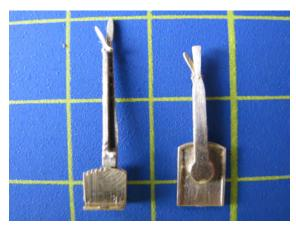
12, Punch the two half etched rivets on part23 (seat bracket) and shape both thebracket and etched seat (part 24) as shown.Fix both in place using adhesive. Thedirection lever can now also be fixed inplace at the rear of the gearbox.
