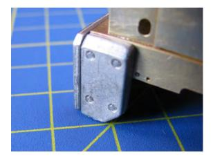
16, Using adhesive, fit radiator grill of choice (part 25 or 25A), small O&K makers plate and white metal filler caps. A small length of 1mm brass L section should be fixed between the footplate and bonnet front.
