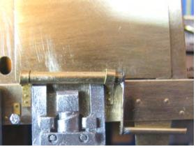
19, The roof (part 32) should now be shaped by gently bending over a piece of bar or an item with a curved edge. Two 34mm lengths of 1.5mm brass L section can then be added to the roof top as shown as rain guards.
