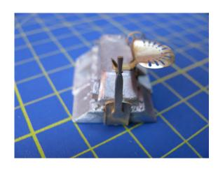
13, The brake lever can now be fixed to the rear of the cab as shown, the now completed gear box, seat etc can also be fixed in place. A small amount of white metal may require removing to allow access for the 8BA nut.
