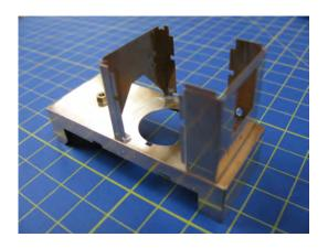
2, There are two alternate bonnet roofs (4 and 4A), one with an exhaust opening and one without. Chose which one is required and punch all 10 rivets prior to folding. Fold to shape as shown taking great care to use a minimum of solder (a tight fit is required when placed onto parts 2 and 3). Solder or glue part 5 (engine access cover) in place and use .45mm brass rod to create the small handle situated at the front top of the bonnet.
