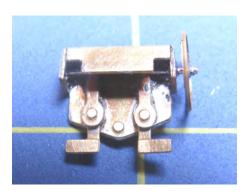
6, Take the two main white metal parts of the gearbox, clean off any flashing and fix together using adhesive as shown. Add handle (part 22), which should be secured in place by drilling a small hole and inserting a short length of .33mm brass wire. The small oval shaped access cover (seen just in front of the seat to the right) should be be fixed as shown.
