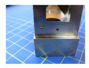
The bonnet roof should now slide over the half etched tabs on parts 2 and 3, once happy all is square it can either be fixed in place or left loose to allow access. It should overlap slightly (by half the thickness of the brass sheet) as per the prototype.
