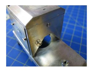
5, Punch the 3 half etch rivets on part 13 and fold to shape as per photo A. Part 14 should be fixed as shown in photo B with parts 15 and 16 overlaying (photo C). Parts 17 and 18 should overlay parts 15 and 16 (photo D). A small length of .45mm brass rod should be passed through the two holes on part 13 and part 21 (speed control hand wheel) and fixed as shown.
