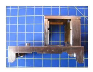
3, Fold part 6 (rear cab cover) to shape and solder in place using the location slots on part 1. Select which bonnet access covers to use (either 7 or 7A) and fix T handles (x 4) in place. The larger of the O&K makers plates can be soldered in place now or glued in place later. The access covers can then be soldered or glued into place spanning parts 2 and 3 (a small gap should be visible just above and below covers when fixed).
