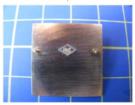
4, Part 8 (x2) should be soldered into place in the location slot provided on part 1 (sloping side to the rear of the locomotive). Open up the slots on part 9 (x 2) and solder the chequer plate steps (2 x part 10) into place. They can then be fixed into the location slots again on part 1.
